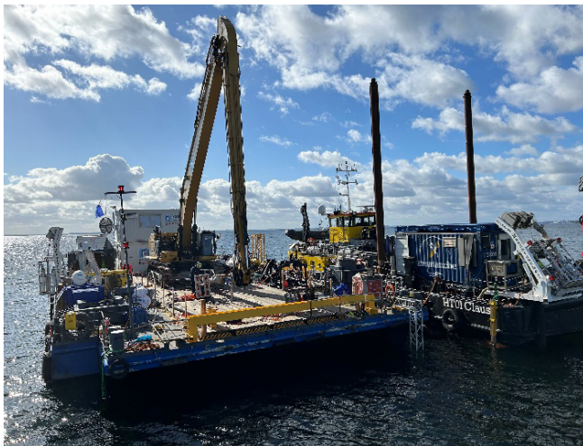
A jack-up barge in Lübeck Bay, Germany, during munition clearance operations in summer 2024 (Photo: GEOMAR).
