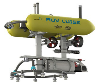
AUV for high-resolution photo surveys. (Photo: Köser, et al. 2024)
