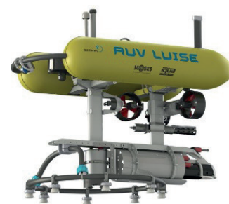
AUV for high-resolution photo surveys. (Photo: Köser, et al. 2024)
