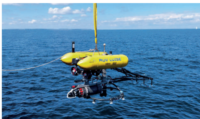
AUV with attached magnetometer. (Photo: Marc Seidel / GEOMAR)
