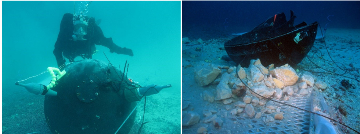
Figure 3: A sea mine disposal by low-order deflagration. Left: Pluton™ deflagration charges placed on the mine shell. Right: After disposal, where large chunks of explosives are visible and no crater. Photo: Norwegian Naval EOD Command.
