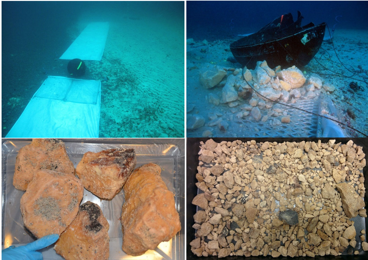
Figure 6: Set up of the low-order experiment and chunks of explosives after disposal of a US MK6 mod 4 sea mine. Photo: FFI and the Norwegian Naval EOD Command.
