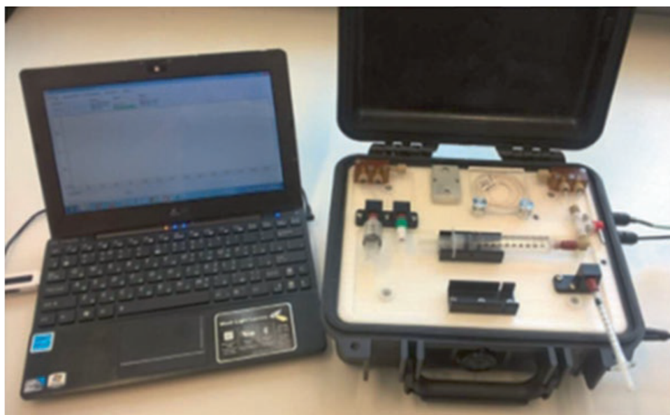
Figure 4 A portable CE-C4D instrument (Fig. after Söderström et al., 2018 ).
