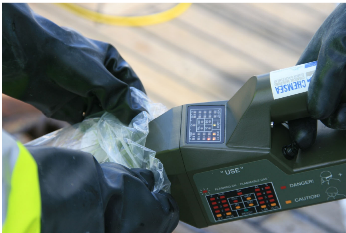
Figure 2 The automatic chemical detection device (AP4C) (Photo by Marita Ljønes).
