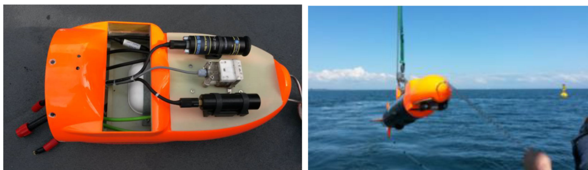
Figure 5. Fraunhofer electrochemical sensor deployed on a SeaCat AUV (Atlas Electronics; images from Fraunhofer ICT, 2018). (Left) Sensor (white box) mounted on the AUV head. (Right) Deployment of AUV with sensor in the Baltic Sea.
