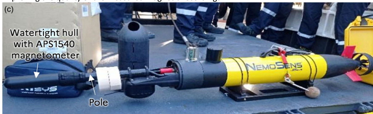
Figure 4. NemoSens Mini-AUV with an APS1540 fluxgate magnetometer attached to the nose of the vehicle (Image from Oehler et al., 2024).
