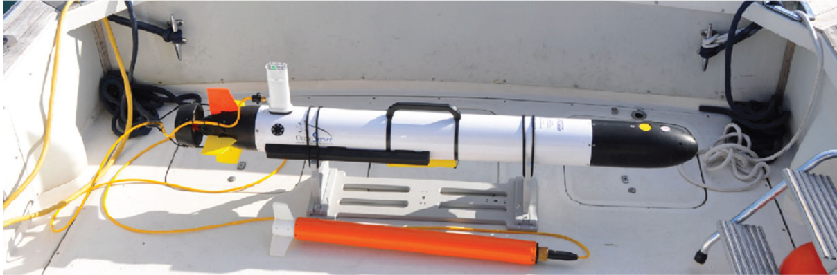
Figure 5. Iver2 AUV with Explorer Magnetometer from MarineMagnetics (Copyright-MarineMagnetics, Canada)
