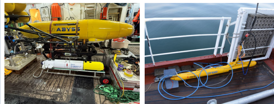
Different size AUVs equipped with the SSS systems and towed system
