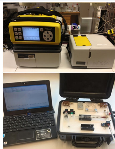
Examples of equipment used on-board (Griffin G510, HAPSITE Portable GC-MS, CE-C'D) (source: Szubska; Jędruch)
