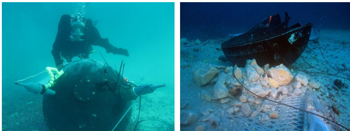
A sea mine disposal by low-order deflagration. Left: Pluton™ deflagration charges placed on the mine shell. Right: After disposal, where large chunks of explosives are visible and no crater. Photo: Norwegian Naval EOD Command
