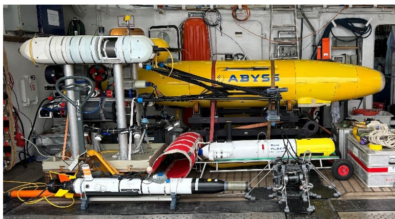
Four different AUVs onboard of RV ALKOR (AL628, March 2025). The AUV in the front left is from IOPAN. Next to AUV work, sediment samples at previously investigated locations were taken (image shows Jacek Beldowski, PI from partner IOPAN).
