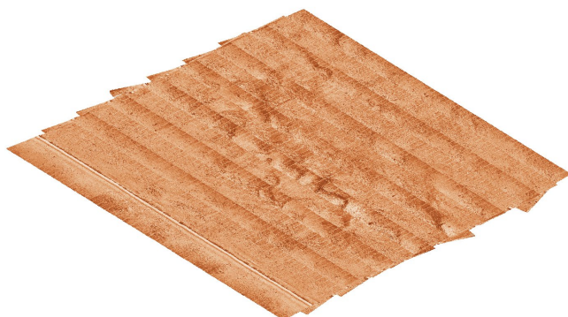
SSS Data from AUV Sparus II Albert automatically processed using side-scan tools during AL644.
