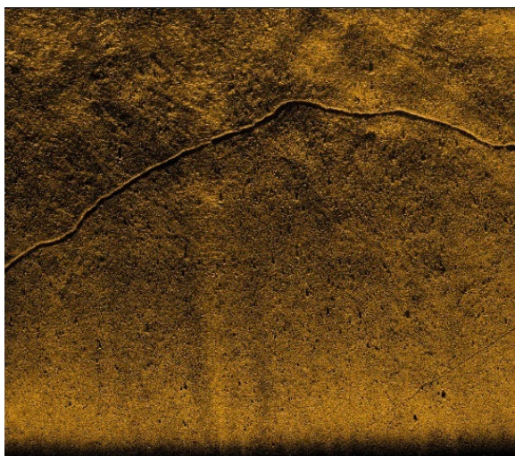
Figure 23 SAS image taken at 9 m water depth, 6 m altitude. The image size is 160 m along-track and 140 m in range. The dynamic range is 40 dB. Left: June 19, 2009. Right: June 28, 2009.
